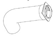
Insert the window unit without its closure cap into the window. Insert the round fitting into the retractable hose and insert the retractable hose with the round fitting into the window unit.
