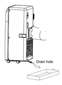
This appliance automatically vaporises condensate in cooling mode.
