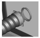
Insert the assembled hose into the back of the air conditioner.
