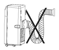
When the air conditioner is not being used, disconnect the hose and fit the closing cap.
